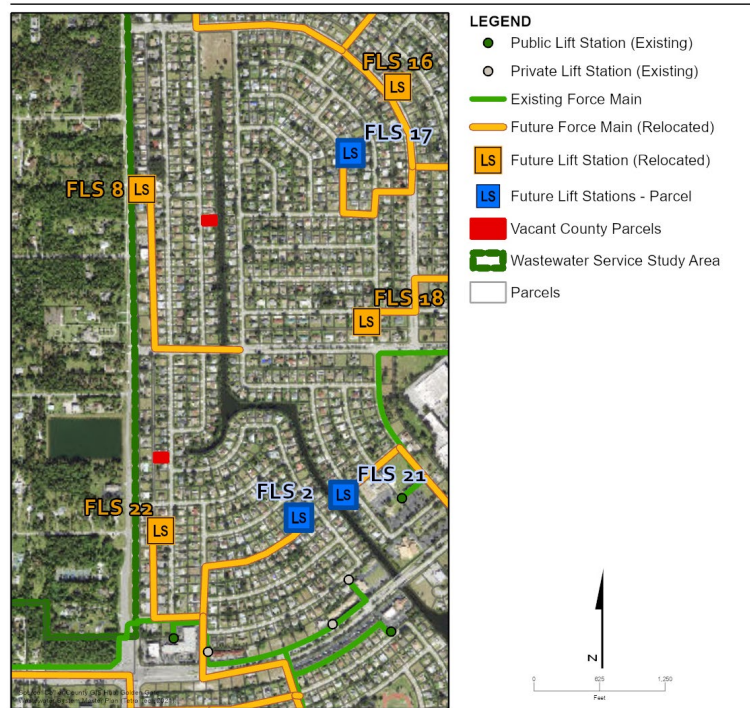
Figure 5. Alternate Future Lift Station Sites
